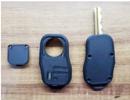
Mobi battery compartment
